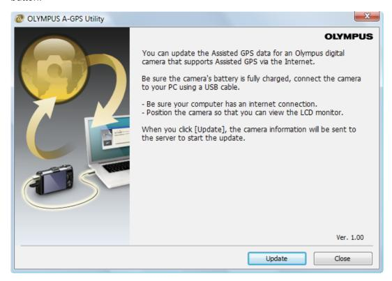
**3** The latest Assisted GPS data will be downloaded from the server and transferred to the camera. After that, the Assisted GPS data on the camera will be updated.
